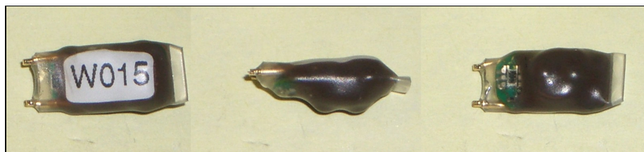
Model: Intigeo-W30A9-SEA 15x5x4mm, 0.45g, 12month battery (e.g. small wader leg)
