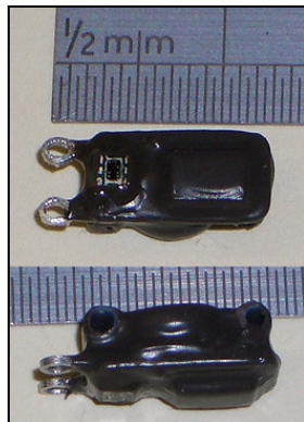
Model: Intigeo-W50B11-DIP 12x5x5.5mm, 0.48g, 15month battery (e.g. passerine back)
