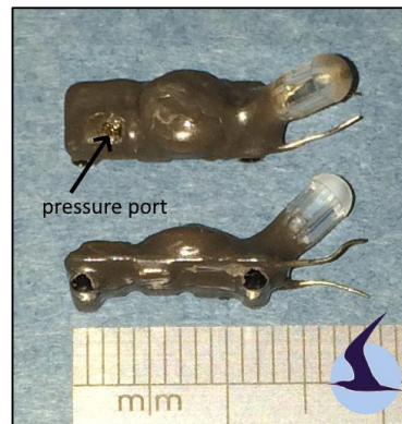
Model: Intigeo-CARP30Z11-7-DIP 14x6x4mm (excl pipe, tubes, contacts) 0.49g, 14month battery (e.g. passerine back)
