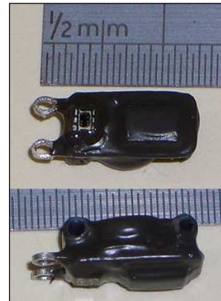
Model: Intigeo-W50B11-DIP 12x5x5.5mm, 0.48g, 9- 13month battery (e.g. passerine back)
