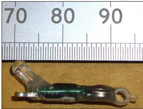
Model: Intigeo-P55B1-7 20x6x3.5mm excluding stalk, 0.60g, 9-13month battery (e.g. passerine back)
