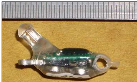
Model: Intigeo-P65C2-7 16x6x6mm excluding stalk, 0.74g, 1-2yr battery (e.g. passerine back)
