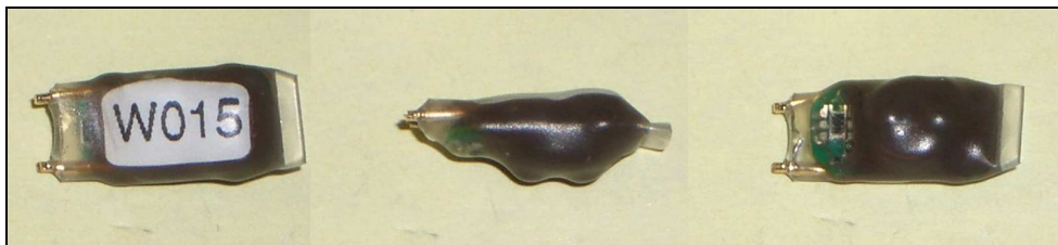
Model: Intigeo-W30A9-SEA 12x5x4mm, 0.45g, 6-8month battery (e.g. small wader leg)
