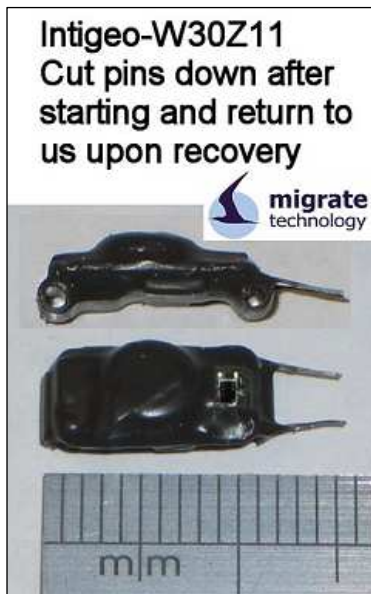
Model: Intigeo-W30Z11-DIP 12x5x4mm, 0.32g, 6- 8month battery (e.g. warbler back)
