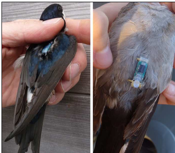
Left: Intigeo-W55B1 (thin package, 1mm loops and tube for harness mounting) copyright Lyndon Kearsley. Right: Intigeo-W65C2-7 (2mm loops and tube used with leg loop harness) copyright Alex Jahn.
